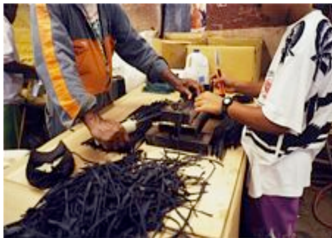
Figure 10. Assembling leather-wrapped wire strapping / Palmwood®. Pacific Green went so far as to phase out the use of toxic glues in their furniture, switching to metal wiring wrapped in natural leather. A close-up of solid Palmwood flooring with a natural wax finish.
